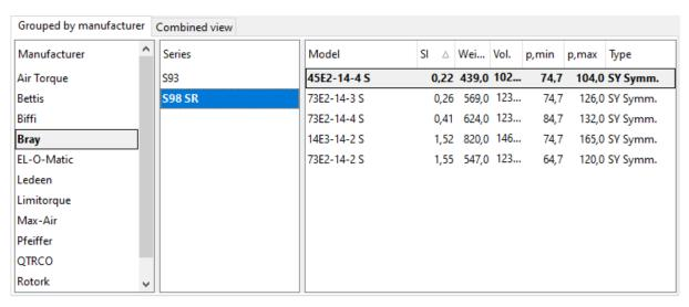
Or use a combined view showing you the suitable devices from your preferred vendor list, ordered by the Suitability Index (SI) - a key performance indicator (KPI) quantifying how closely assembly meets application requirements).
