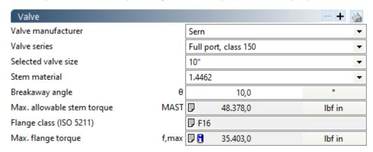
But in our case, we selected the valve from the vendor database (which is constantly growing) and automatically get all we need. Based on that information, the torque requirements are calculated.
