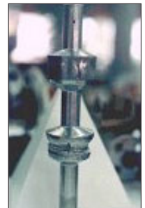
Fig. 20: Damage due to flashing if p_2 \ll p_v and v_2 \gg 60 m/s.
