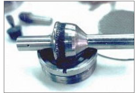
Fig. 19: Typical damage due to cavitation if pressure differential > 20 bar. Feedwater control valve mismatched for start-up 70 to 1 bar.
