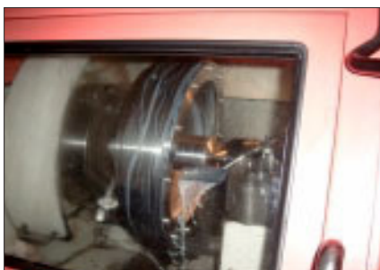
Fig. 43 LTR 43 triple eccentric seat ring manufactured by LEUSCH to achieve a rangeability of 1 to 100.
